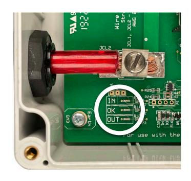
The TX LED indicates there is power on the antenna. It will flash when the charge pulse is on and scanning for tags. The brightness will change while tuning, getting brighter as it gets closer to 134.2 kHz.
