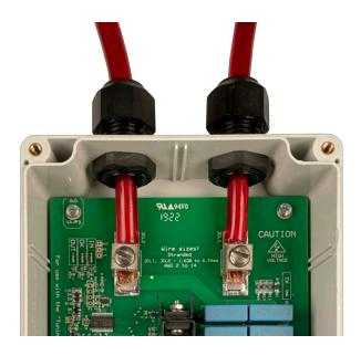
If the wires are too thin and the grips cannot seal, short pieces of rubber cord can be used to fill the gap.
